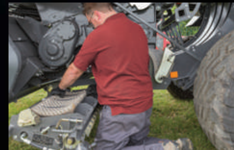
▲ Ample accessibility offering straightforward knife removal
